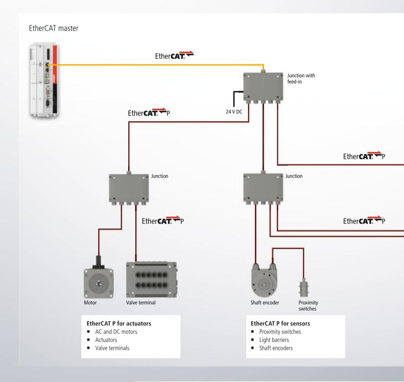
With EtherCAT P, Beckhoff combines communication and power in a single 4-wire standard Ethernet cable. The 24 V DC supply of the EtherCAT P slaves and of the connected sensors and actuators is integrated:  $U_{\rm S}$  (system and sensor supply) and  $U_{\rm P}$  (peripheral voltage for actuators) are electrically isolated from each other and can each supply a
