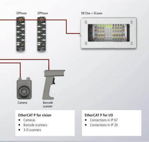
into the wires of the 100 Mbit/s line, enabling the realisation of a highly cost-effective and compact connection. EtherCAT P offers benefits both for connection of remote, smaller I/O stations in the terminal box and for decentralised I/O components locally in the process. A connector family was specially developed for EtherCAT P, in order to prevent
